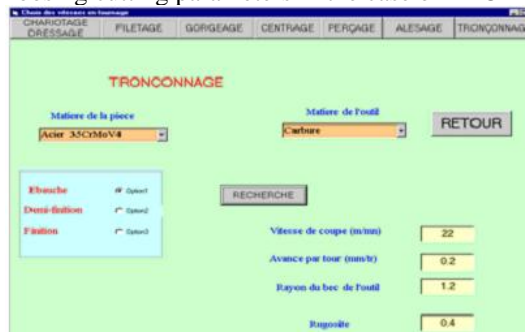
Fig 12. Help in choosing cutting parameters in the case of CUTTING
