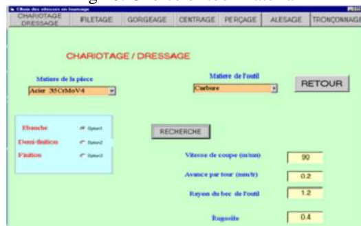
Fig 11. Help in choosing cutting parameters in the case of TROLLING/DRESSING
